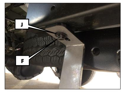
6 Repeat steps 1-5 on the right side using the right bracket (C). If your van has a rear tow hook, it will need to be removed.
