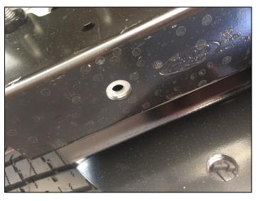
Insert bolt (F) with washer (J) into the left bracket (B) as shown. Then start the M10 thread plate (I) onto the bolt.
