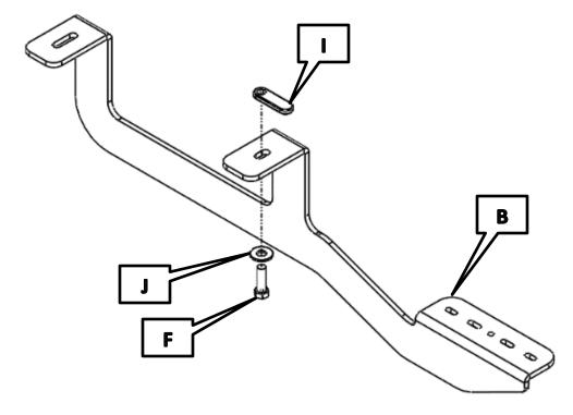
Insert the M10 thread plate while still attached to the bracket into the rear mounting location of the vehichle. Then align the bracket with the front mounting location.
