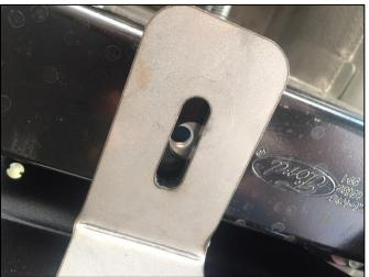
Insert bolt (F) and washer (J) into front mounting location. Do not fully tighten at this
